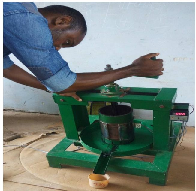
Figure 1. Pictorial view of the screw press during pressing operation.
